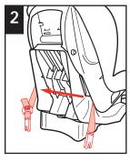
Adjuster MUST be on the left side of child restraint as shown. DO NOT twist belt.
